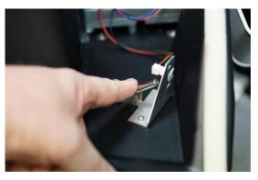
To test the emptying mode, fix the levelling arm in activated position. Depending on program version, it will take about 1-4 days end then the toilet will activate and show "time to empty" in the display.
