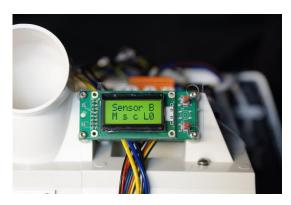
Push the top of the compost level arm forward, check the service menu and when the sensor is activated the letter should change to a capital "C"
