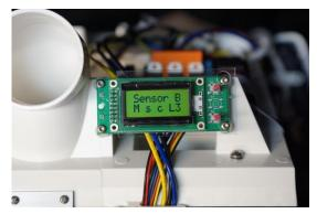
To check the compost sensor; the letter "c" in the service menu is the compost level arm and when the level is too low the sensor is deactivated and there should be a small letter.
