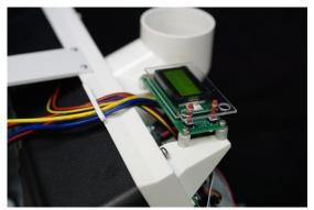
After a few seconds you will enter a service menu. Move forward by pushing button A. At Sensor B check the letters on the second line. The letter L has a digit behind it and when the tray has no liquid, it should read L0.
