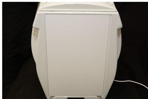
3. Pull off the cover plate and remove the insulation.
