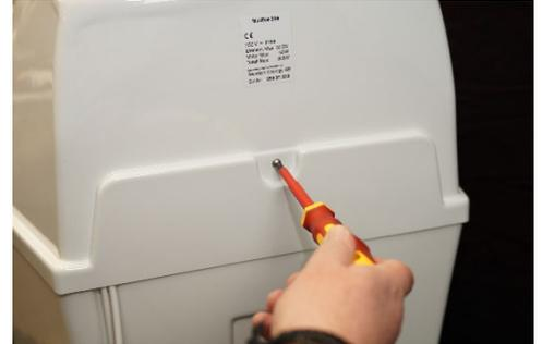
Remove the handle by removing the shear pin from it (15e).
