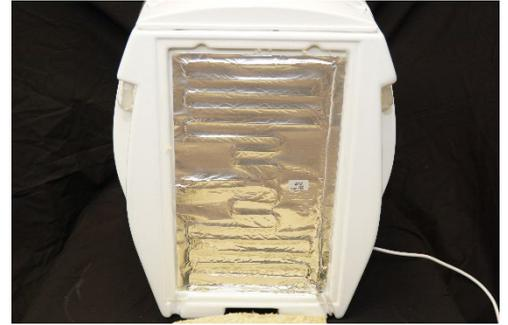
6. Put the insulation in place as well as the cover plate. The cover plate is provided with a double-sided tape.
