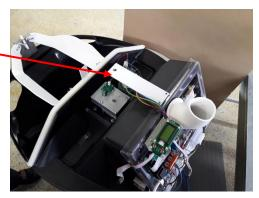
3. Disconnect the contact on the circuit board (sensor).
