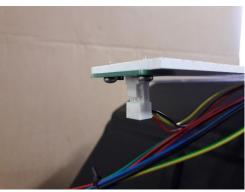
4. Unfasten the bracket and turn it upside down and unfasten the old circuit board (sensor).
