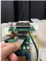
Remove the 4 screws holding the display pcb.
