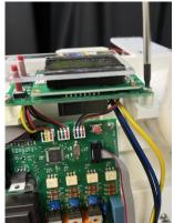
Make sure to keep the 4 rubber distances in position when removing the display.
