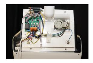
Remove the connection cable for the display
