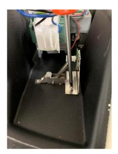
3. Remove the switch on the circuit board.
